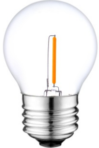
352-19 M45mmN 78mm 2700K 80Ra 150lm 360° 2W (≈16W) E27 220-240VAC EC A+
