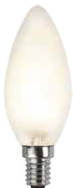
350-13 M35mmN 94mm 2700K 80Ra 320lm 360° 4W (≈30W) E14 220-240VAC EC A+
