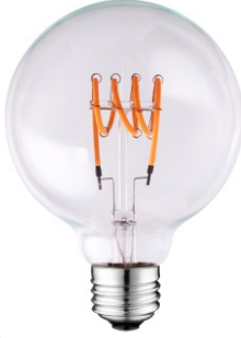
351-04 M95mm N138mm 2700K 80Ra 200lm 360° 4W (≈37W) E27 220-240VAC EC A+
